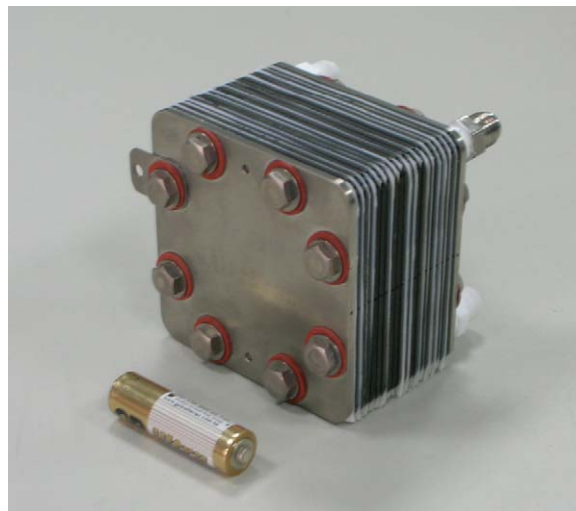
Fig. 1. An experimental 18-cell bipolar plate stack.
